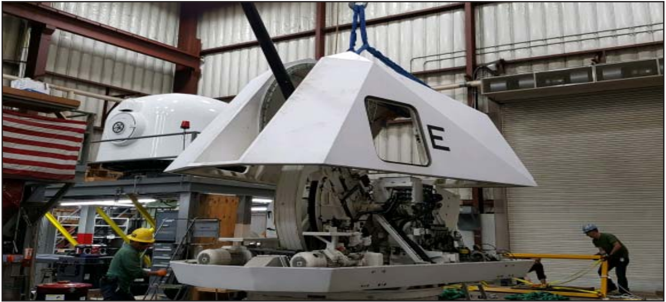
National Security Cutter’s MK 110 57mm gun overhaul
