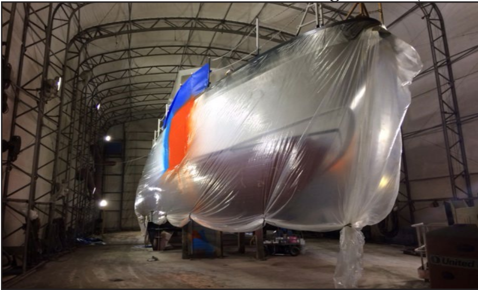
The patrol boat POMPANO undergoes painting during its 60-day planned maintenance under the Coast Guard's 87' Recurring Depot Availability Project (RDAP). POMPANO is the 4th Phase II RDAP vessel and will report to its new homeport in Tybee Island, GA upon completion of work at the Yard.
