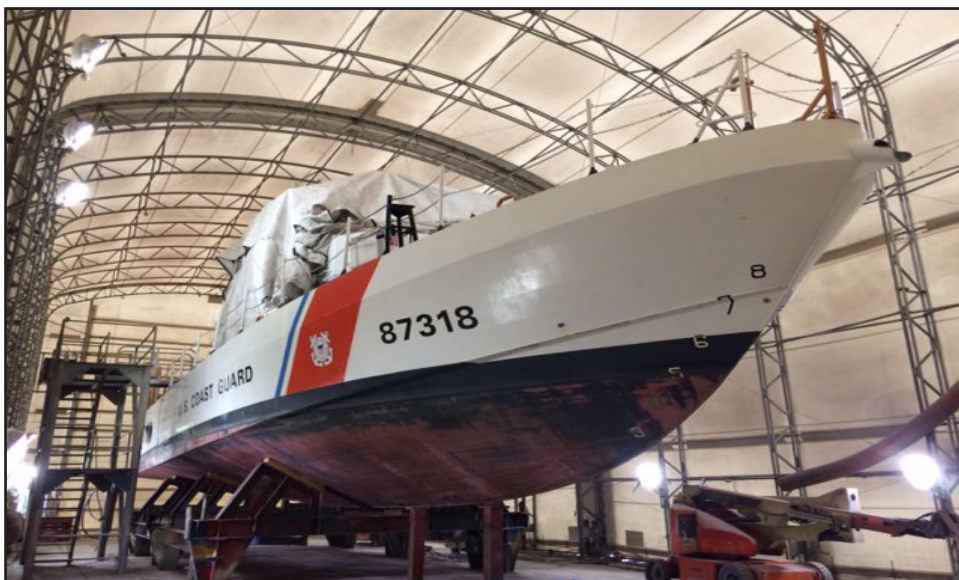
The Yard prepares the 87' patrol boat BLUEFIN for blasting as it undergoes a 60-day planned maintenance under the Recurring Depot Availability Project (RDAP). BLUEFIN is the 5th Phase II RDAP vessel and will report to its new homeport in Virginia Beach, Virginia after completing RDAP.
