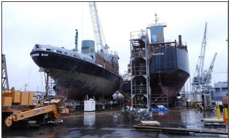
The Yard delivered the THUNDER BAY (left), a 140' ice breaking tug, in mid-November after completing a 12-month Service Life Extension Project (SLEP) under the Coast Guard's In-Service Vessel Sustainment Program. Work was completed on time and under budget and involved replacement of major hull, mechanical, electrical and electronic systems. THUNDER BAY's new homeport is Rockland, Maine.
