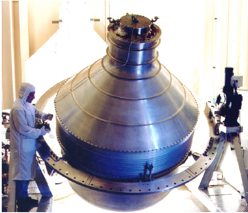
The probe rests inside a 645-gallon, 9-foot tall dewar filled with liquid helium.
