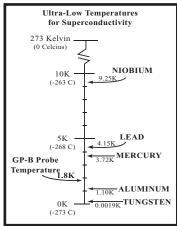
Gravity Probe B applied the London moment phenomenon to its experiment by coating its four fused quartz gyroscopes with a sliver-thin layer of niobium (1270 nanometers thick), a superconducting metal. As predicted by the "London moment", when each gyroscope spins, the superconducting
