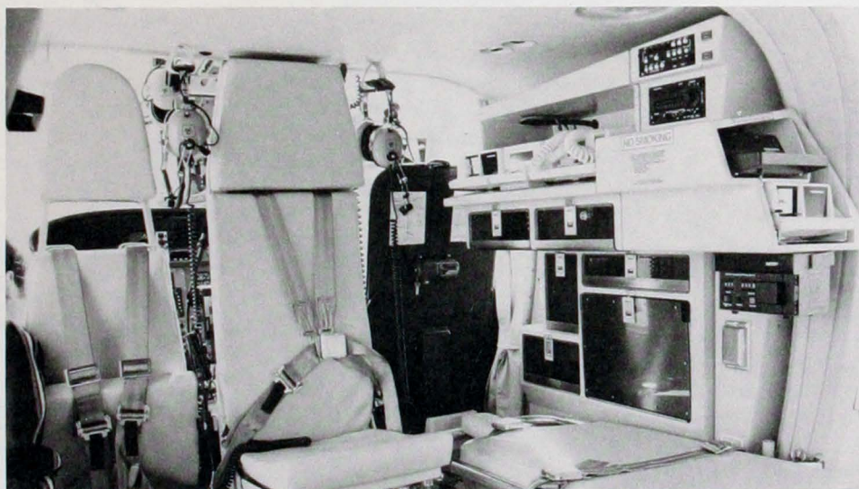
The secondary patient litter on the right side (pilot side) of the helicopter is next to medical equipment and medical radio communication equipment.
