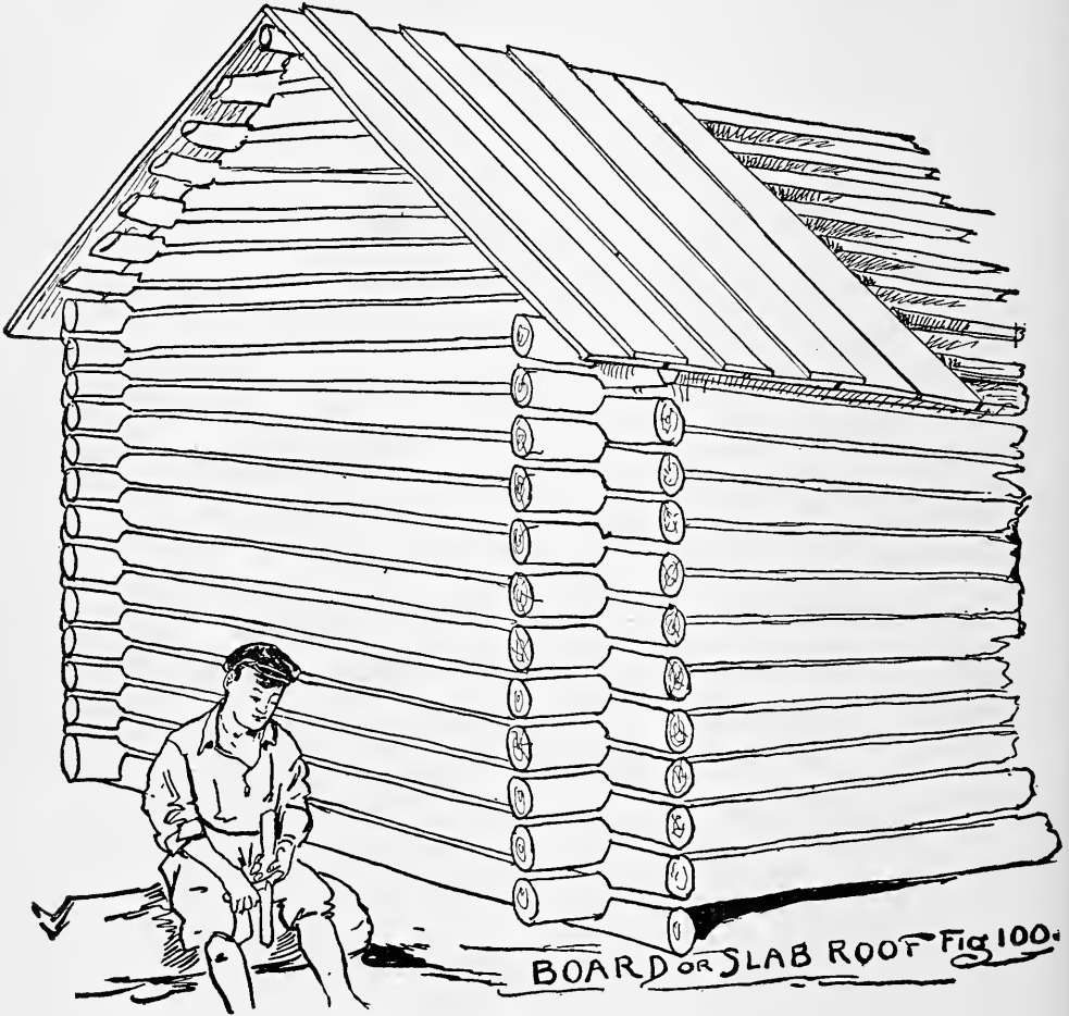
FIG. 100.—Board or Slab Roof.
