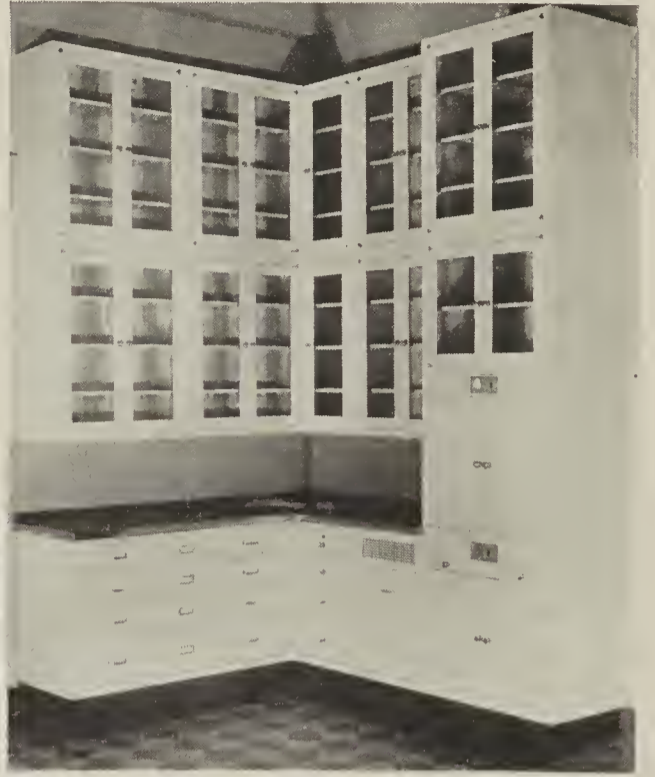
A grouping of units including linen and silver drawers, soiled linen bin, towel dryer, with plate warmer at counter height
