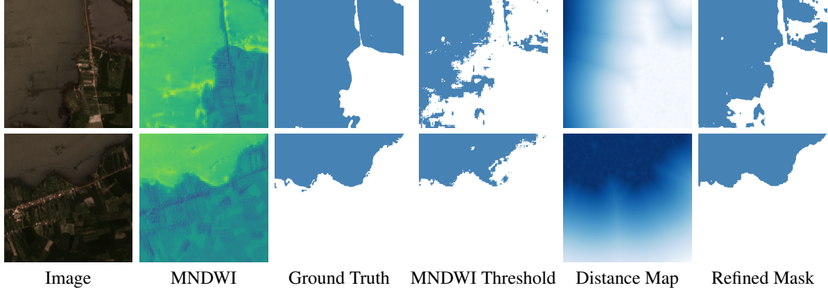
Figure 4: Qualitative results of our refiner on PlanetScope [2]. Our refiner provides better ground truth for the segmentation network without hand-labeled data. Our refiner samples high confidence points from MNDWI used to generate adaptive distance maps, which are then concatenated to MNDWI to make 2 channel input to the refiner. Blue and white predicted pixels represent water and non-water pixels. Best viewed in color and zoomed.
