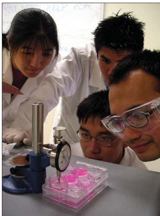
Students in BioE 115 test the mechanical properties of their engineered cartilage Photo courtesy of Terry Johnson
