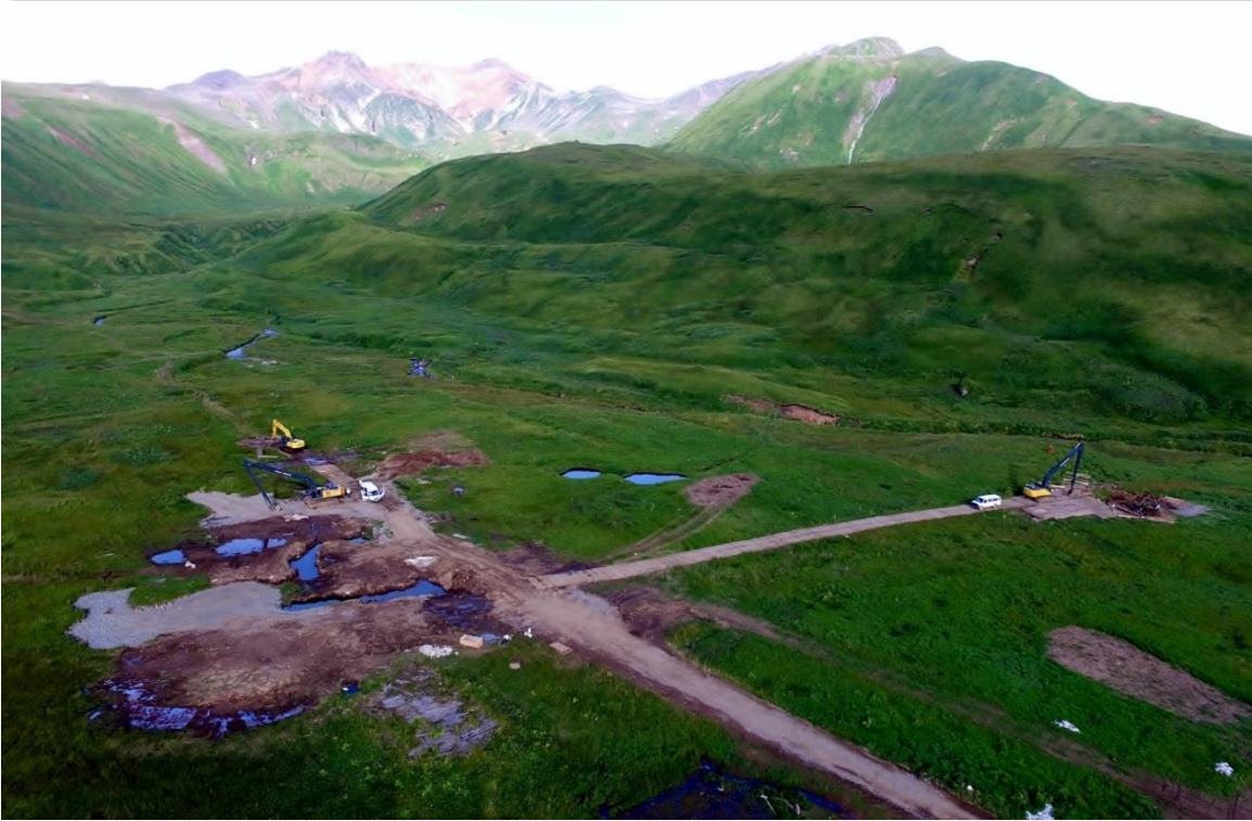
Former Adak Naval Complex, Operable Unit B-2 (OUB-2)-View of Remedial Action Area (RAA) – 01 in Moffet Valley, Adak, Alaska. This is a former open burn/open demolition area for munitions. Note the remnant blast craters. Two long reach armored excavators are visible in the photographs. Note the wooden platforms placed as roadways to minimize impact to the tundra wetlands (Photo/ Abtim)
