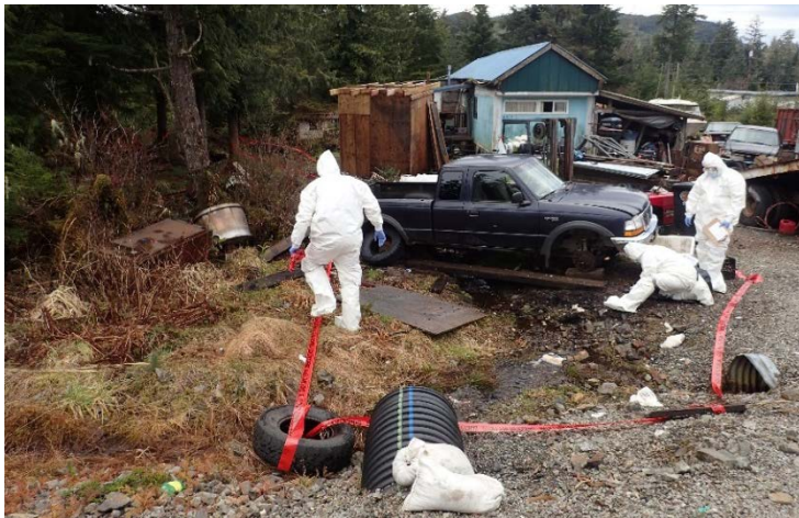
DEC responder collecting soil samples at the site of the transformer oil dumping, February 23, 2016 (Photo/Klawock Fire Dept.)
