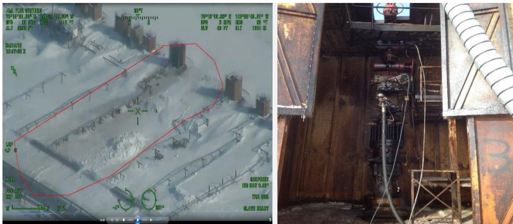
LEFT - Forward looking infrared (FLIR) overflight shows crude spray plume. Crude misting is visible on snow within red line delineated at Well 3, April 14, 2017 (Photo/BPXA) RIGHT - Drill Site (DS) 2, Well 3, showing well house and tree after well was controlled, April 20, 2017 (Photo/DEC)
