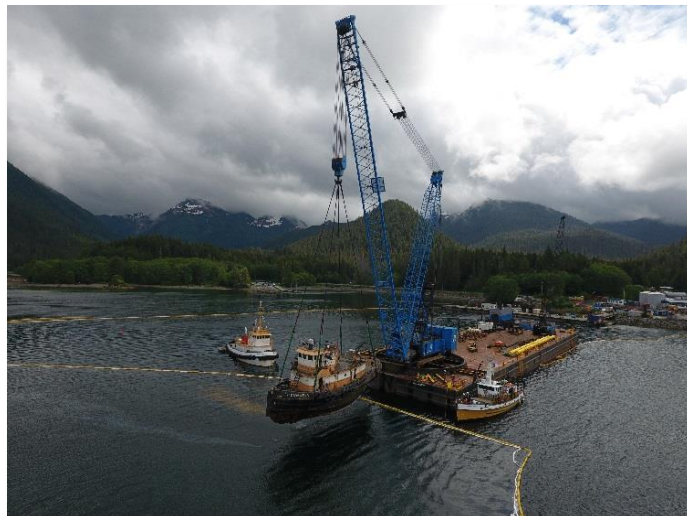
The tug Powhatan is raised from the bottom of Starrigavan Bay. June 12, 2017 (Photo/Samson Tug & Barge)
