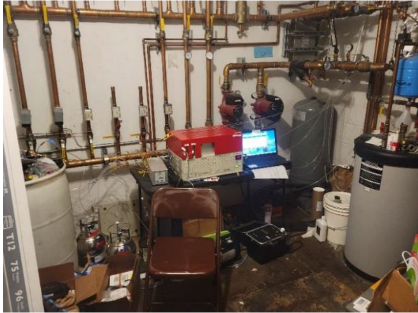
Photo: A portable filed gas chromatogram (GC Unit) operated by EPA ORD staff in the basement of a church in Fairbanks, measuring indoor air contaminants.
