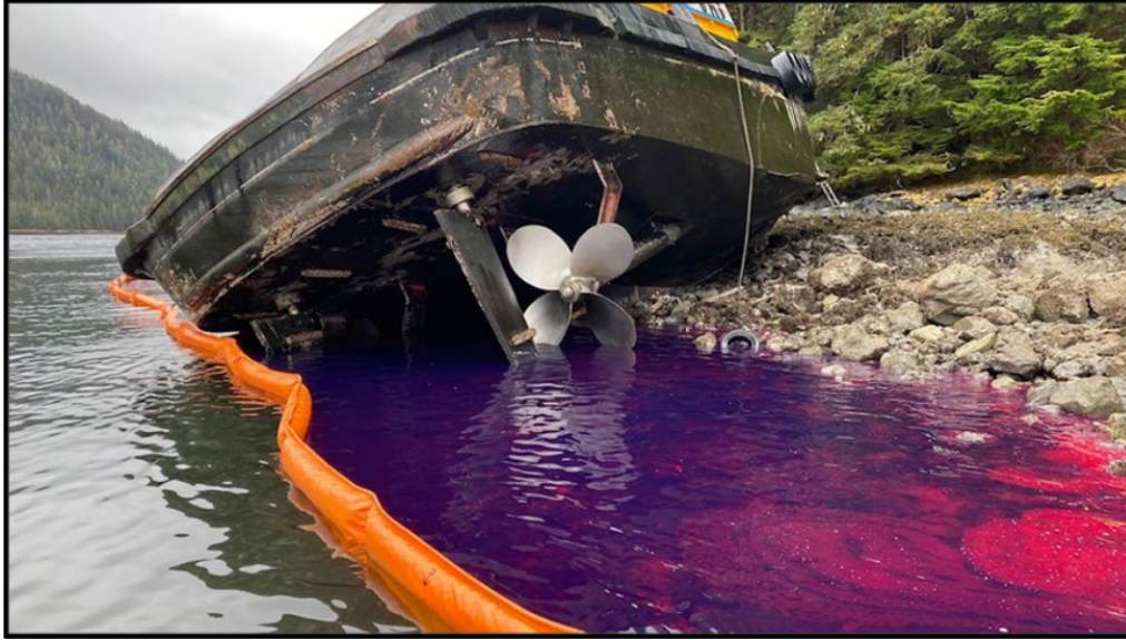
Contaminated boom deployed following the grounding of the tug Western Mariner in Neva Strait on March 21, 2022. Red-dye diesel contained within boom was recovered using skimmers and absorbent materials. (Photo credit Hanson Maritime.)
