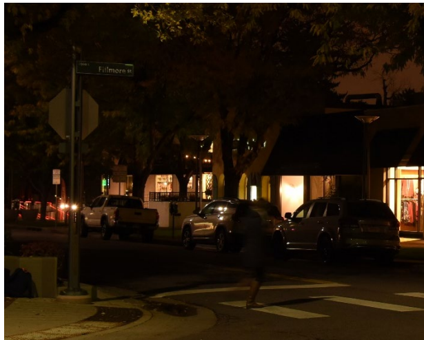
Figure 5-6: Poorly Lighted Crosswalk
