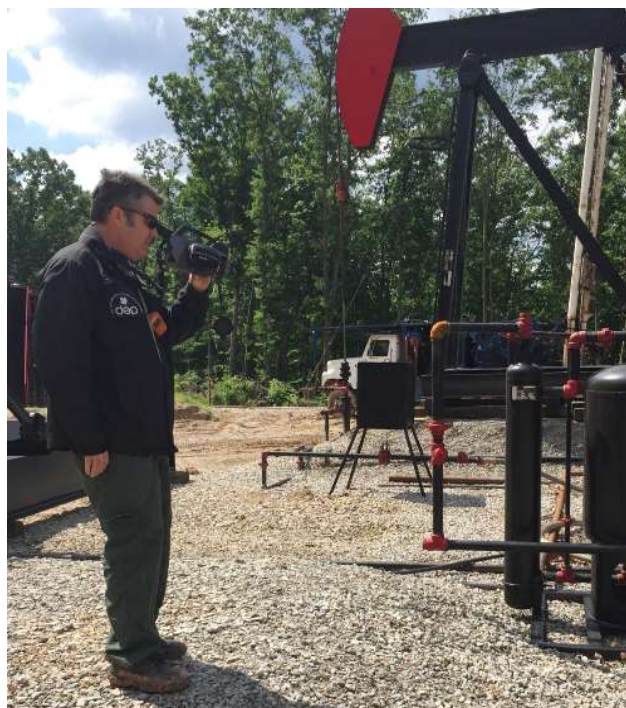
Air Quality inspector using optical gas imaging camera
