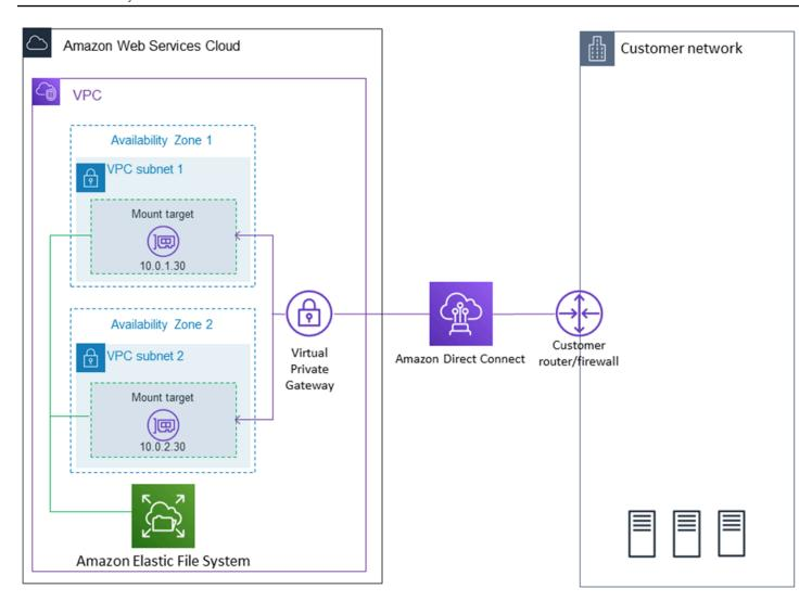
You can use any mount target in your VPC if you can reach that mount target's subnet by using an AWS Direct Connect connection between your on-premises server and VPC. To access Amazon EFS from an on-premises server, add a rule to your mount target security group to allow inbound traffic to the NFS port (2049) from your on-premises server. For more information, including detailed procedures, see Prerequisites.
