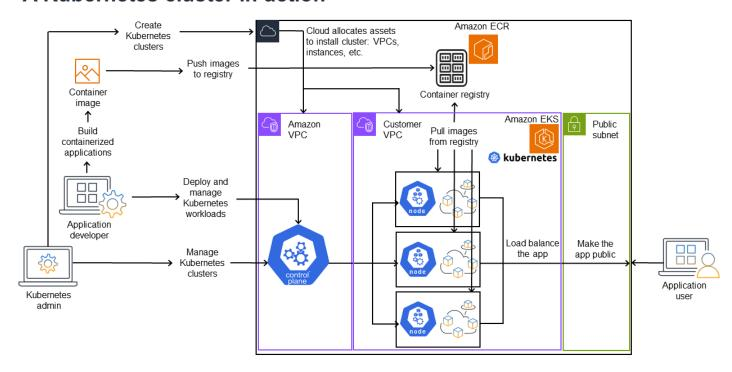
A Kubernetes Admin creates the Kubernetes cluster using a tool specific to the type of provider on which the cluster will be built. This example uses the AWS cloud as the provider, which offers the managed Kubernetes service called Amazon EKS. The managed service automatically allocates the resources needed to create the cluster, including creating two new Virtual Private Clouds
