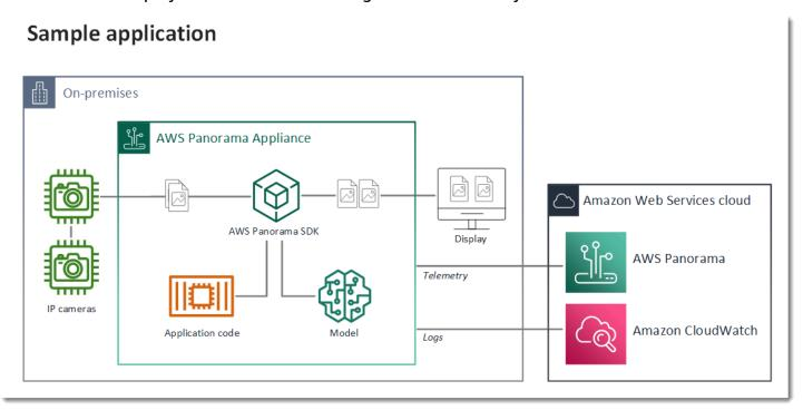
In this example, the application uses the AWS Panorama Application SDK to get frames of video from a camera, preprocess the video data, and send the data to a computer vision model that detects objects. The application displays the result on an HDMI display connected to the appliance.
