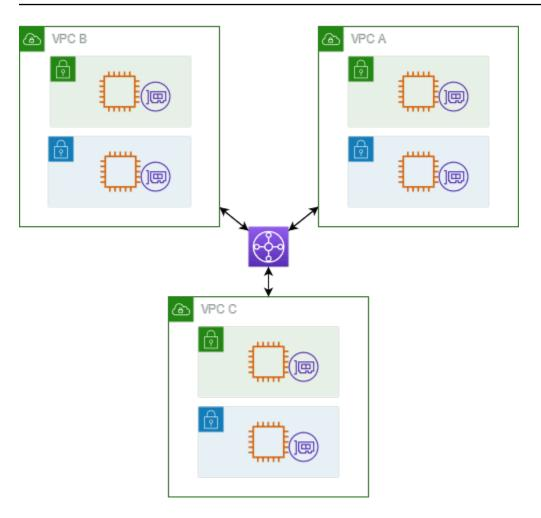
The following is an example of a default transit gateway route table for the attachments shown in the previous diagram. The CIDR blocks for each VPC propagate to the route table. Therefore, each attachment can route packets to the other two attachments.
