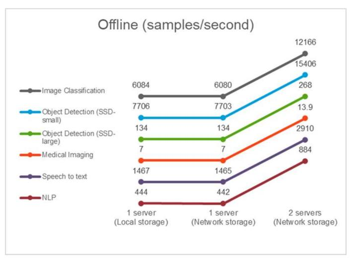
The results show that network storage does not negatively affect the performance—the change is minimal and for some tasks, none is found. When adding the second server, the total bandwidth either exactly doubles, or at worst, the change is less than 1%.
