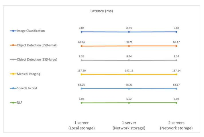
The results show again that the network storage is sufficient to handle the tasks. The difference between the local and network storage in the one server case is minimal or none. Similarly, when two servers use the same storage, the latency on both servers stays the same or changes by a very small amount.
