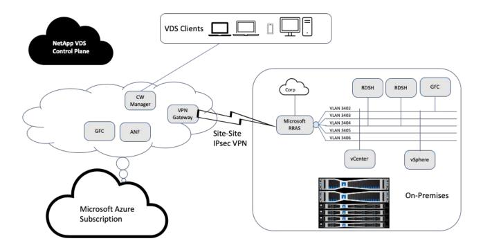
On-premises, we had multiple VLANs for management, remote-desktop-session hosts, and so on. They were on the 172.21.146-150.0/24 subnet and routed to the corporate network using the Microsoft Remote Routing Access Service. We also performed the following tasks:
