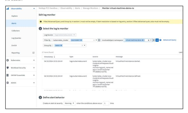
This query provides all the events for the virtual machine in the namespace. (There is only one virtual machine in the namespace). An advanced query can also be constructed to filter based on the event where the reason is "failed" or "FailedMount" These events are typically created when there is an issue in creating a PV or mounting the PV to a pod indicating issues in the dynamic provisioner for creating persistent volumes for the VM.
