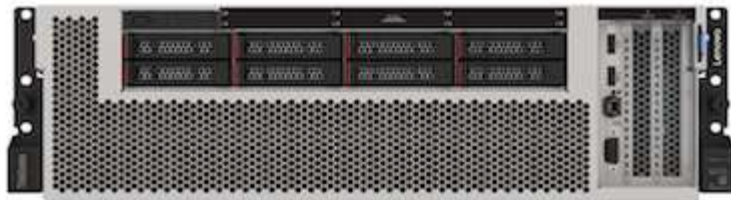
4x SXM GPUs with 8x 2.5-inch HS drives and 2x PCIe I/O slots
