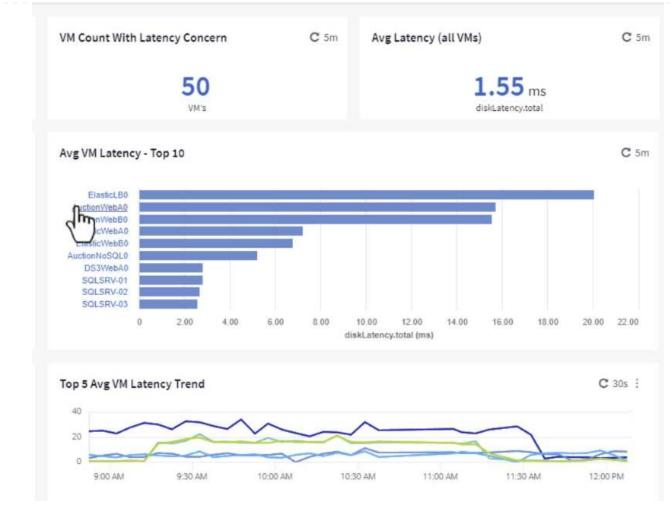
4. The VMs potentially causing workload contention are listed and available. Drill into these VMs performance metrics to investigate any potential issues.
