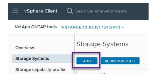
3. Fill out the IP Address, credentials of the storage system and the port number. Click on **Add** to start the discovery process.
