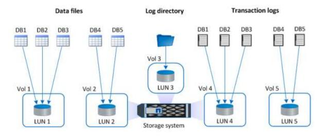
The Log directory is dedicated to SnapCenter to perform transaction log rollup for database recovery. For an extra large database, multiple LUNs can be allocated to a volume for better performance.
