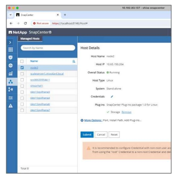
2. Install and configure the storage plugin. From the added host, select "More Options". Navigate to and select the downloaded storage plugin from the NetApp Automation Store. Install the plugin and save the configuration.
