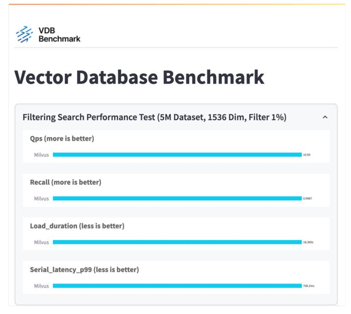
From the performance validation of the standalone Milvus instance, it's evident that the current setup is insufficient to support a dataset of 5 million vectors with a dimensionality of 1536. we've determined that the storage possesses adequate resources and does not constitute a bottleneck in the system.
