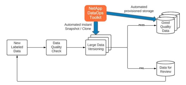
The NetApp DataOps Toolkit complements the data quality-checking pipeline through the use of its nearinstantaneous data cloning technology. Each labeled file must be assessed and compared to the existing labeled files. Distributing these quality checks across various data storage systems ensures that these checks are executed quickly and efficiently.
