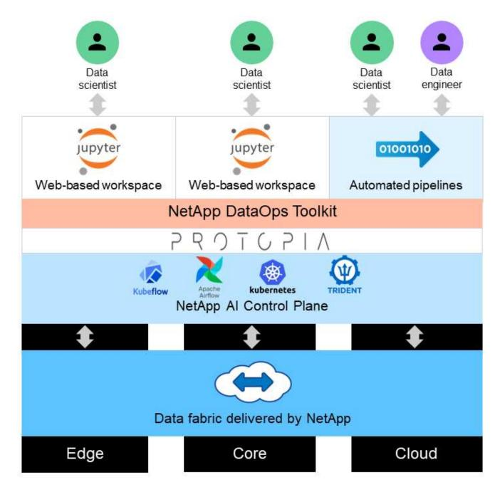
Protopia obfuscation software runs seamlessly on top of the NetApp DataOps Toolkit and transforms the data before leaving the storage server.
