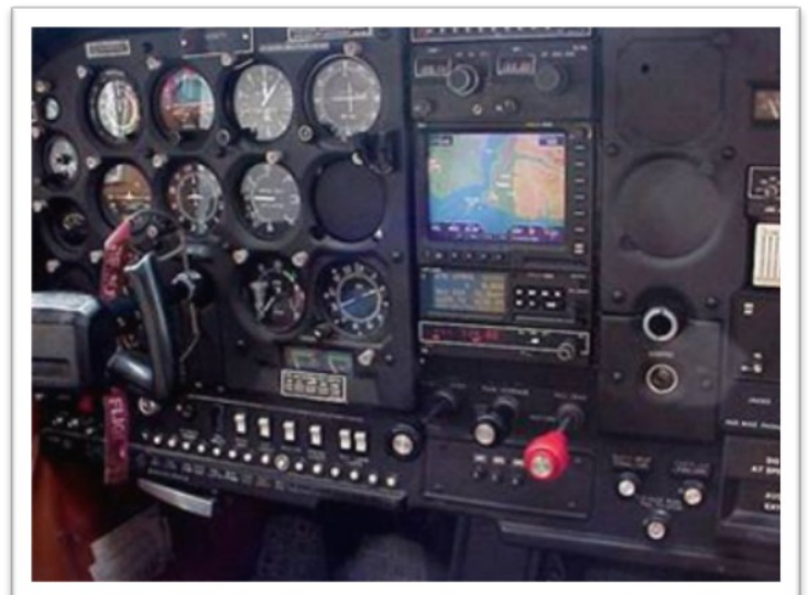
NextGen equipped airplanes have a “moving map” video display screen that shows the pilot his own location relative to terrain, weather, and equipped airplanes in the vicinity.
