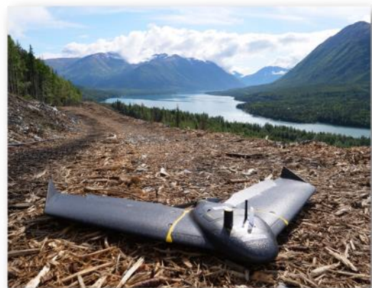
Sensefly Ebee X - looks like a soaring eagle! Wing Span: 45.7 inches; Flight Time: 90 Minutes; Cruise Speed: 25-68 mph; Range: 60 Miles
