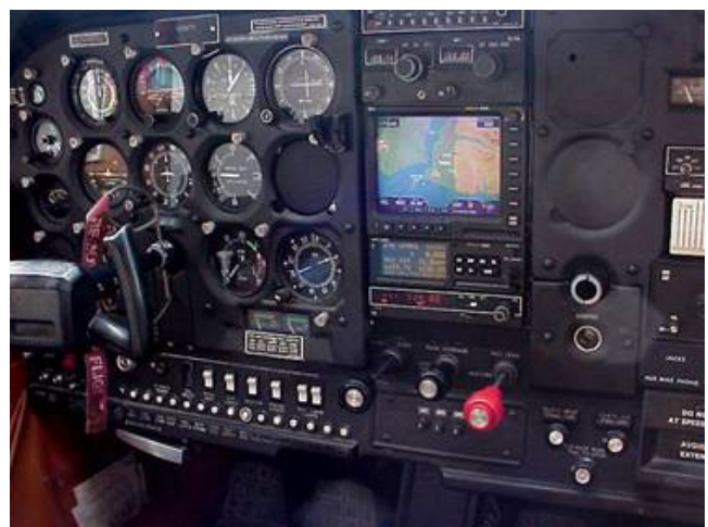
NextGen equipped airplanes have a "moving map" video display screen which shows the pilot his own location relative to terrain, weather, and equipped airplanes in the vicinity.
