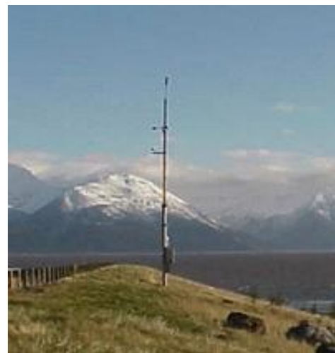
RWIS Installation at Bird Point, Jack Stickel, ADOT&PF
