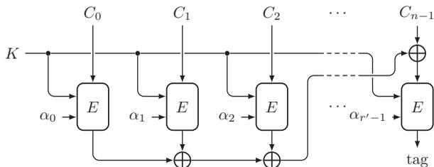
**Figure 2:** tPMAC, the Tweaked Parallel Message Authentication Code.
