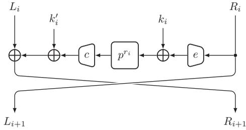
**Figure 1:** Structure of a MATTER Feistel round.
