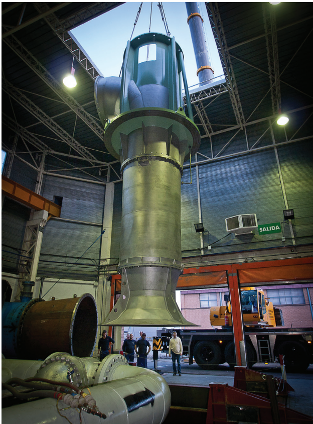
Figure 7: One of five 62 APM circulating water pumps for a plant in Saudi Arabia
