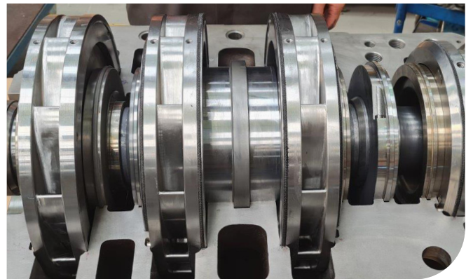
Flowserve designs the runners and nozzles on HDO-TT rotor assemblies (like the one shown above) to match a CFD analysis of conditions stage by stage. (See CFD images below.) This is what we mean by a true-turbine design.
