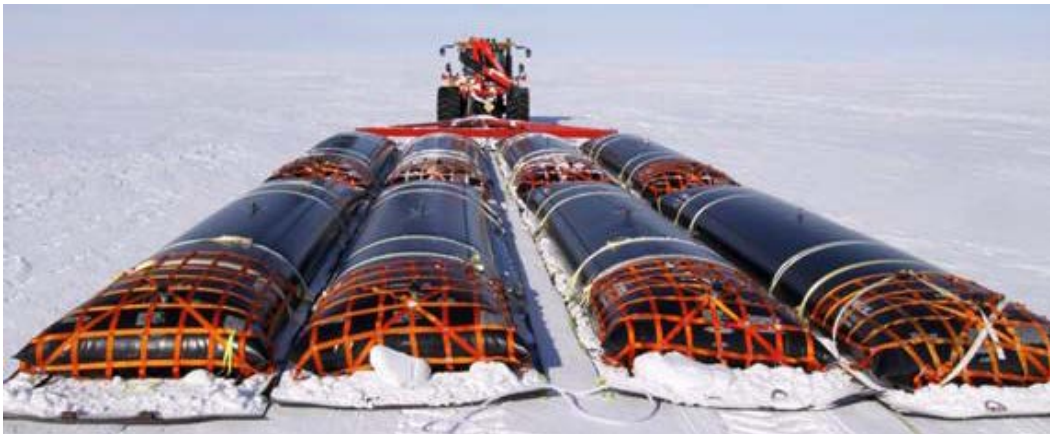
Figure 1. Fuel sleds towed outbound from McMurdo Station to South Pole Station in 2010–11. Each 8 ft wide × 68 ft long × 0.5 in. thick HMW-PE sheet carries two 3000 gal. fuel bladders.
