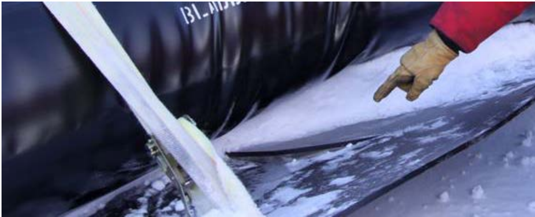
Figure 2. A crack in HMW-PE sheet during outbound trip to South Pole in 2010–11.
