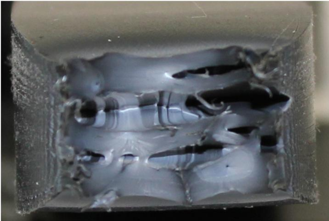
Figure 16. Splitting and crazing of Vendor A HMW-PE at failure surfaces of a new, unused specimen ( upper ) and a field specimen ( lower ) tested at -40^{\circ}\text{C} and 20 in./min.
