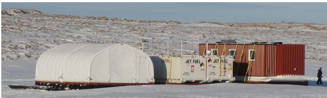
Figure 5. GrIT14 ARCS carried a prefabricated berthing module ( red ) along with two empty steel fuel tanks and food, tools, and miscellaneous payload inside tent enclosures.
