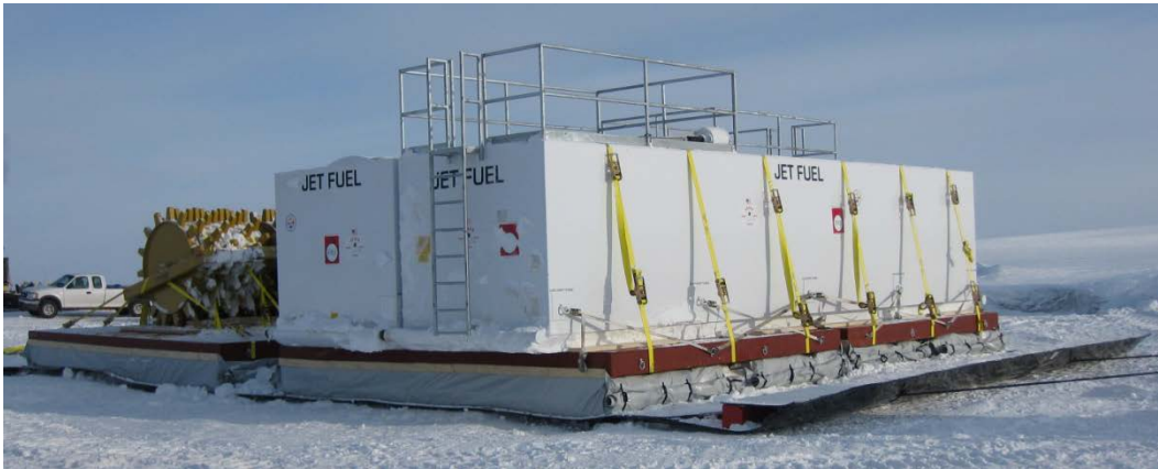
Figure 4. GrIT12 ARCS loaded for the outbound trip to Summit Station. The two front sleds carried two 24,000 lb empty steel fuel tanks. One rear sled carried a 14,000 lb roller-packer while the other rear sled carried food and tools inside a tent enclosure. As with its bladder sleds, GrIT towed the assembly of four adjacent HMW-PE sheets through a ski-nose spreader bar.
