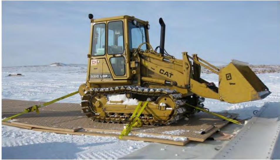
Figure 9. Assembled Dura-Base cargo sled, consisting of eight interconnected tan mats, connected to the large spreader (via lifting straps) and loaded for a test run.
