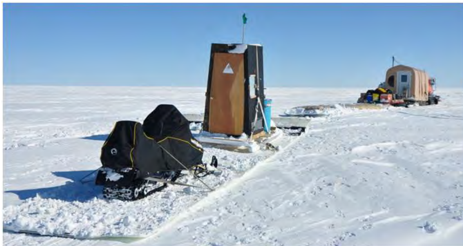
Figure 4. Sled train behind Tucker SnoCat in 2010 (right to left): wannigan, orange sled with camp supplies, 3000-gal. bladder sled, short spreader, spare HMW-PE sled carrying outhouse, and snowmobile (photo courtesy Robin Davies).
