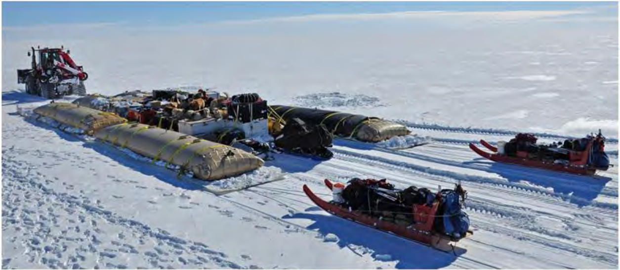
Figure 5. Case Quadrac towing full load of dual-3000-gal. bladder sleds on either side of a Dura-Base cargo sled. The left-side bladder sled included electric blankets under both bladders, while both bladders on the right-side sled were wrapped in black covers. The photo (courtesy Robin Davies) shows Go North dogs and sleds catching a lift en route to NEEM.
