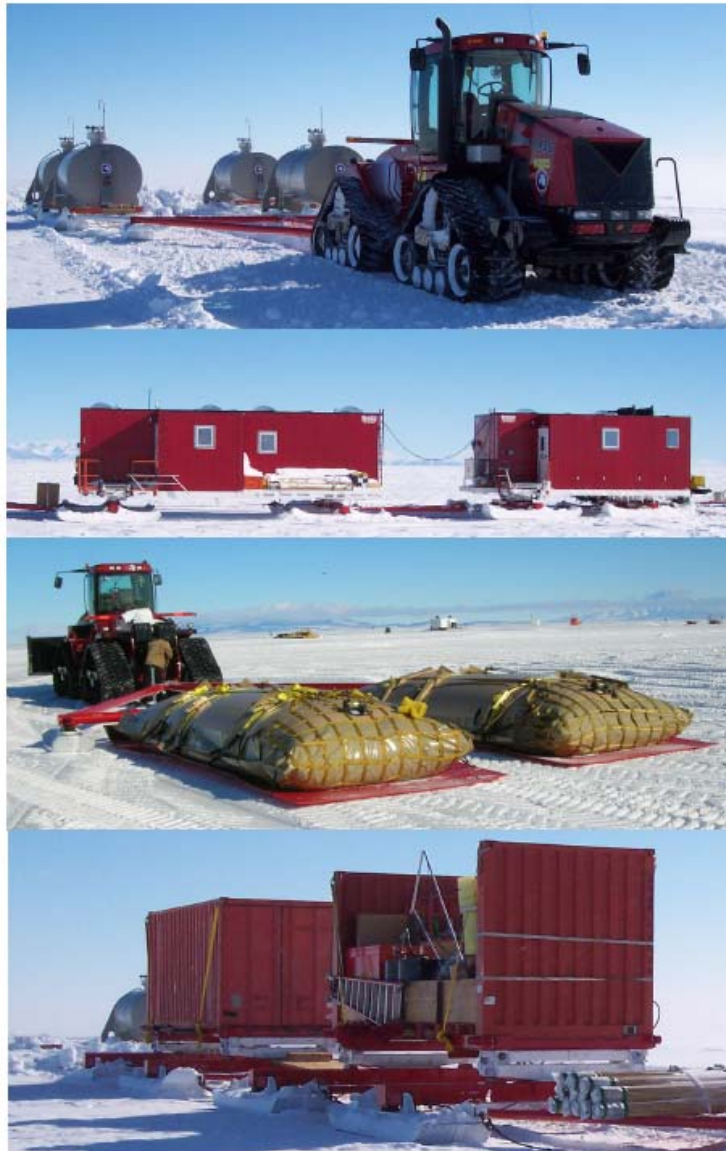
Figure 2. Example tractors and sleds used on the South Pole Traverse (top to bottom): Case STX450 tractor pulling four fuel tanks in 2 \times 2 configuration; living and energy modules for fleet support; newly developed fuel-bladder sleds; cargo sleds.
