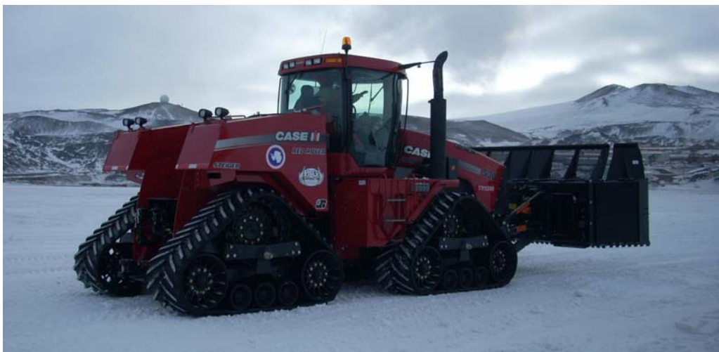
Figure 3. Case STX530 with plowing blade and dual auxiliary 300-gal. rear fuel tanks.
