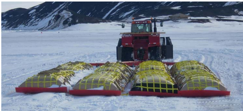
Figure 4. SPT bladder sleds assembled for the 2007-08 season. Each sled consists of two 3,000-gal. bladders strapped to a welded sheet of UHMW. Here, four sleds are laced together to form a group of eight bladders for towing behind a single tractor using a spreader bar.
