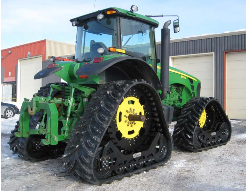
Figure 15. John Deere 8530 tractor equipped with Soucy tracks prior to over-snow traction tests in Drummondville, Quebec, in February 2009.
