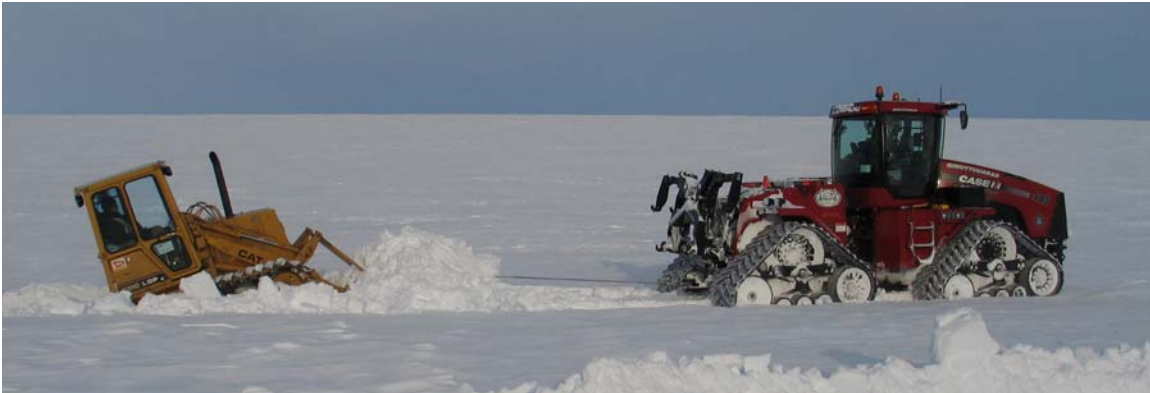
Figure 10. Case Quadtrac, in its lightest configuration, towing the Caterpillar 931 during drawbar tests. The 931 had difficulty bringing the Case to a halt even with its tracks locked and bucket buried.
