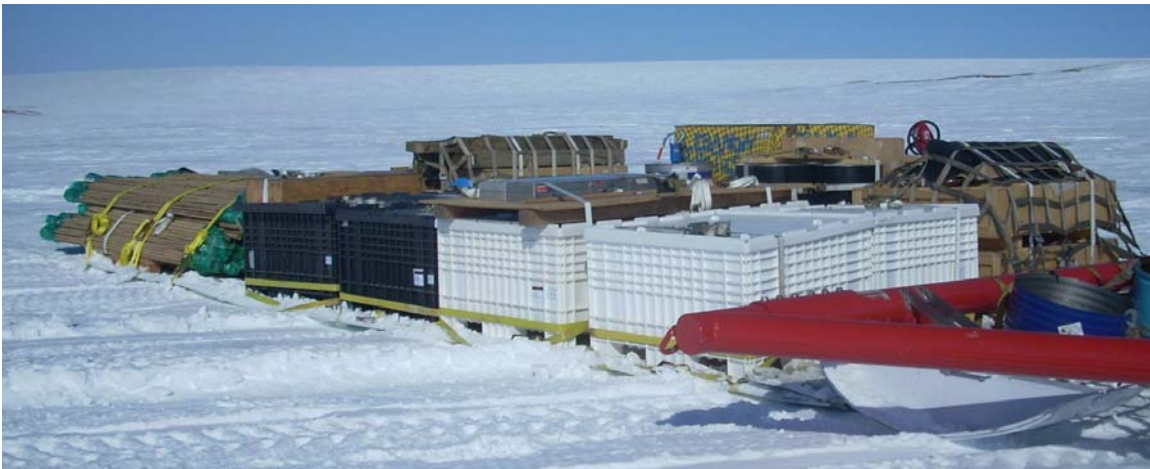
Figure 6. Two flexible cargo sleds, each consisting of boxes, pallets or bulk cargo strapped directly to a flexible sheet of HMW-PE.
