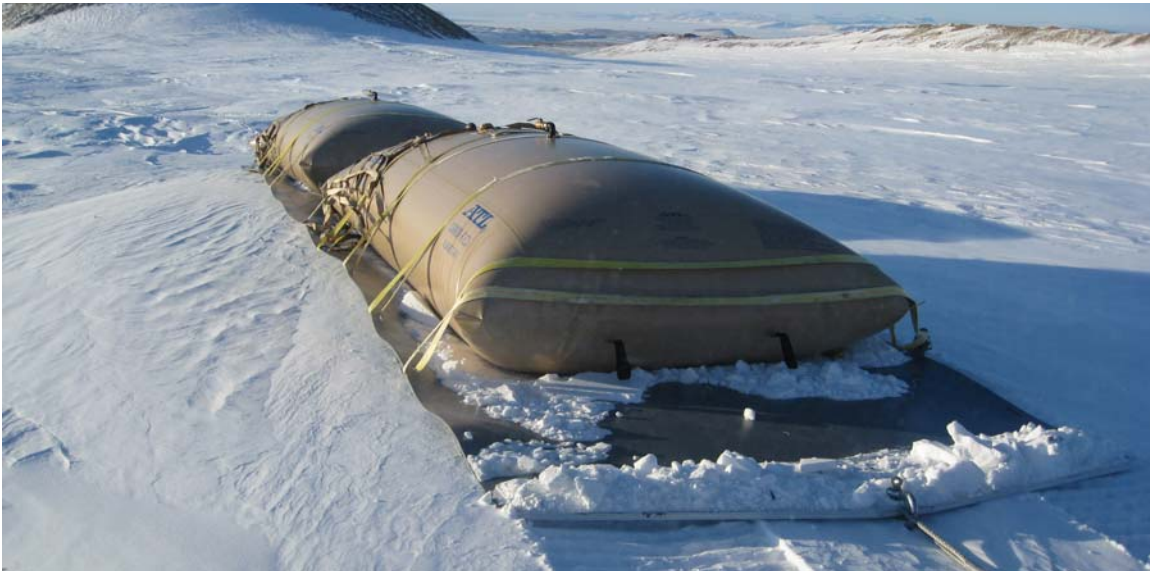
Figure 11. Bladder sled consisting of two welded sheets of UHMW-PE and two 1500-gal. bladders.
