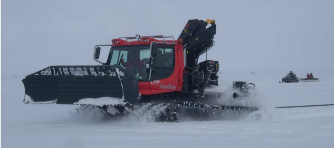
Figure 14. Pisten-Bully 300 towing four GrIT08 bladder sleds at NEEM. Despite an impressive DBP/W = 0.61 , the tractor was power-limited at 6 mph and its operator expressed reliability concerns about towing all day under these conditions.
