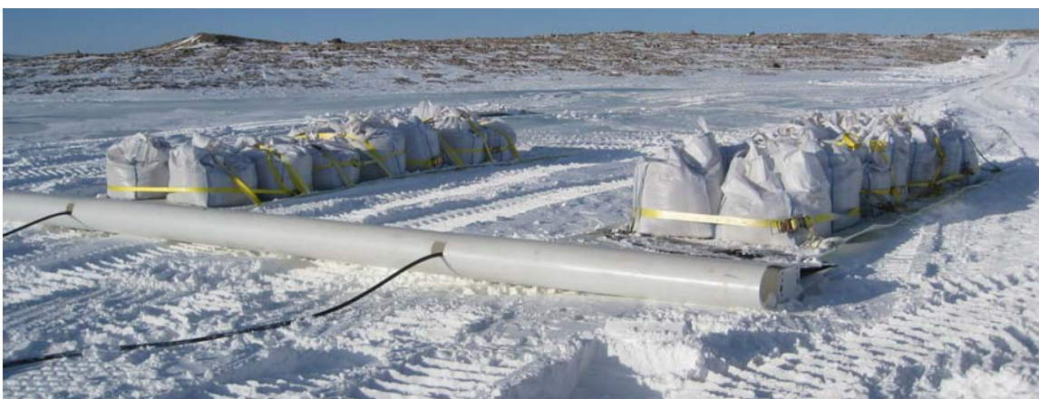
Figure 12. New spreader bar consisting of square-section steel tubing wrapped with a sheet of HMW-PE to form a curved nose and to support bladder- and cargo-sled tow plates.
