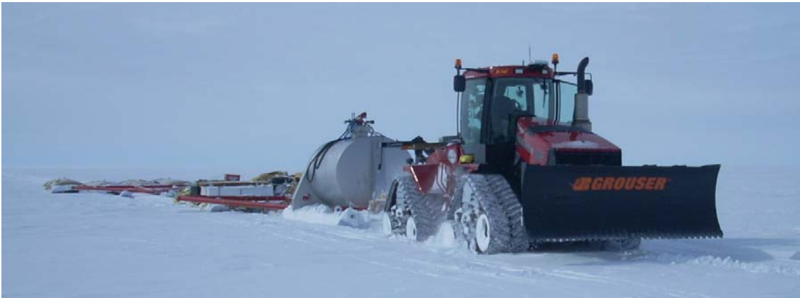
Figure 2. Case Quadtrac towing all GrIT08 heavy sleds: a steel fuel tank, two flexible cargo sleds on a spreader bar and four flexible bladder sleds on a spreader bar.
