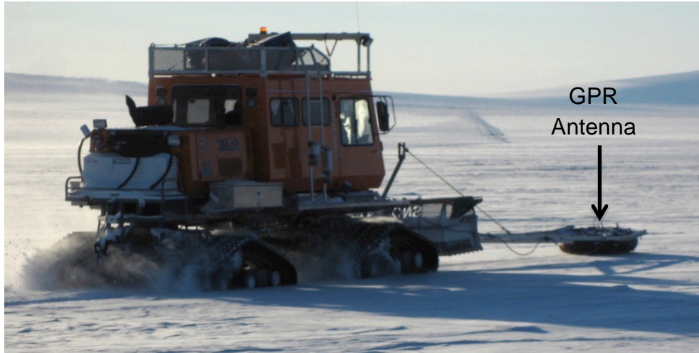
Figure 3. SCAT's manual-survey vehicle consists of a Tucker Sno-Cat equipped with a GPR antenna on a 6 m long boom. An operator interprets the GPR signals in real time to detect the presences of underlying crevasses while a driver and navigator guide the vehicle along the prospective route.
