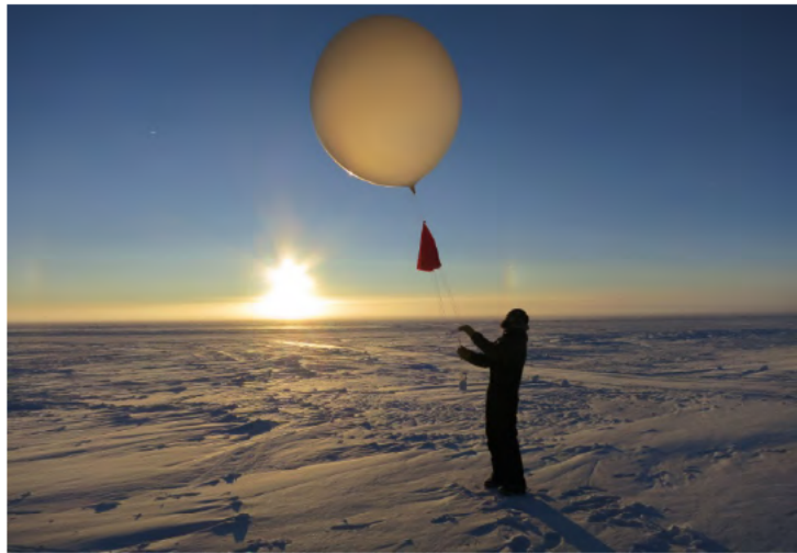
Science technician preparing for an Integrated Characterization of Energy, Clouds, Atmospheric state, and Precipitation at Summit radiosonde balloon release.
