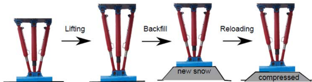
Figure 12. Sketch of the lifting sequence for Neumayer III Station (Rotthäuser and Jagolski 2010).
