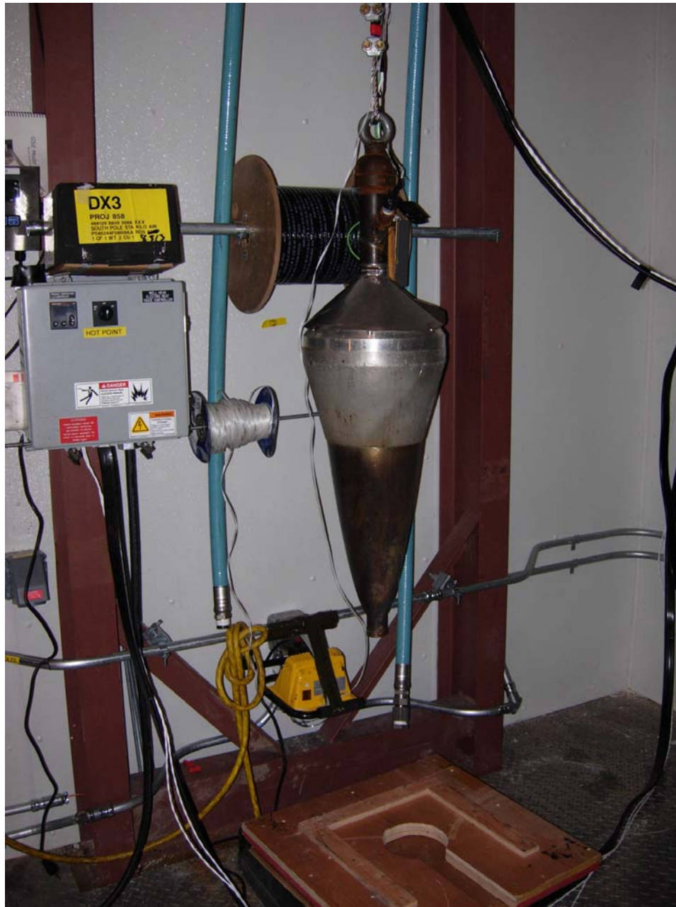
Figure E.4. Hot point drill used to establish the initial well shaft for the Rodwell at South Pole (photo obtained from NSF/RPSC South Pole Project files).
