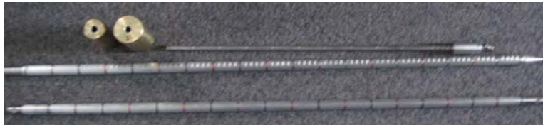
Figure B1. Rammsonde Cone Penetrometer shown with 1-m extension, guide rod, and drop weights.
