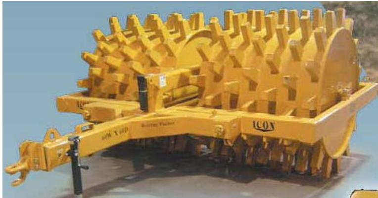
Figure 5. Sheepfoot roller similar to the one delivered to Summit Station in 2012.
