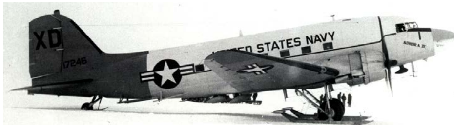
Figure A1. R4D aircraft on skis. (Photo taken from US Navy, www.bluejacket.com .)
