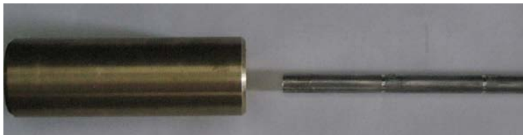
Figure B3. Pick a weight and slide it down the guide rod (left). Unless the skiway is very hard, use the 1 kg weight.
