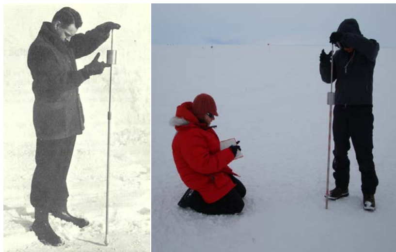
Figure A15. Left: Rammsonde penetrometer in 1973 (Clark et al. 1973). Right: Rammsonde use in 2009.
