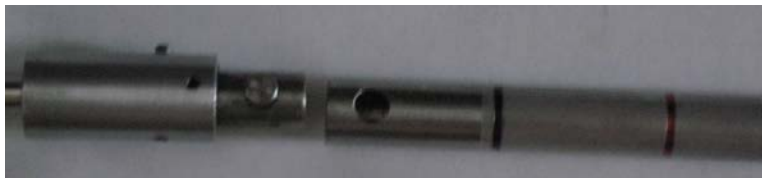
Figure B2. Connect the guide rod (left) to the main shaft of penetrometer (right).
