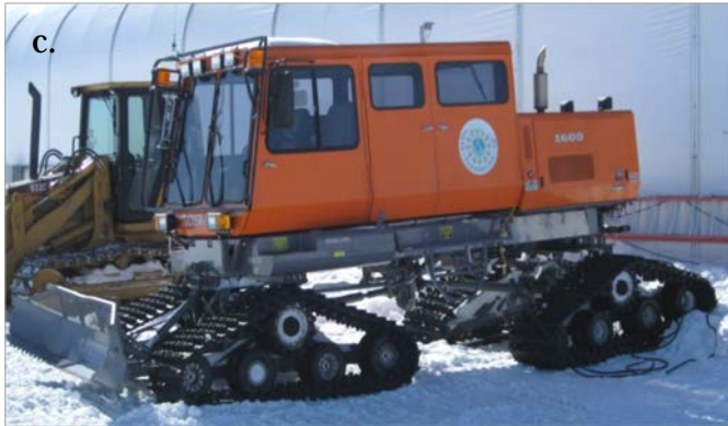
Figure A-1 (cont.). Equipment currently available at Summit includes (a) a Case 335 Magnum tractor, (b) a Cat D6M bulldozer, (c) a Tucker 1600, (d) a sheepsfoot, (e) a landplane, (f) a 24 ft beam drag, (g) a maxi groomer, and (h) a harrow.
