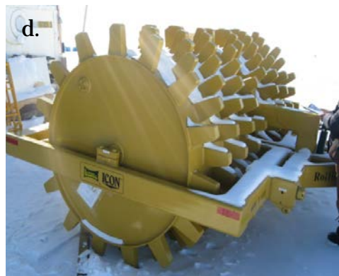
Figure A-1 (cont.). Equipment currently available at Summit includes (a) a Case 335 Magnum tractor, (b) a Cat D6M bulldozer, (c) a Tucker 1600, (d) a sheepsfoot, (e) a landplane, (f) a 24 ft beam drag, (g) a maxi groomer, and (h) a harrow.
