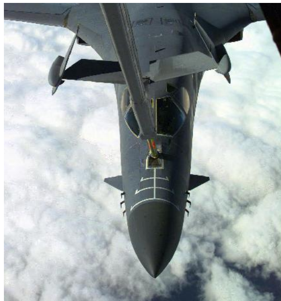
Figure 2: B-1B Lancer Refueling From a KC-135 Using Boom and Receptacle Method
