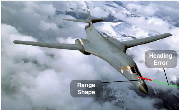
Figure 10: Illustration of Range Shape (red) and Heading Errors (green), Visual Position Sensing Simulation
