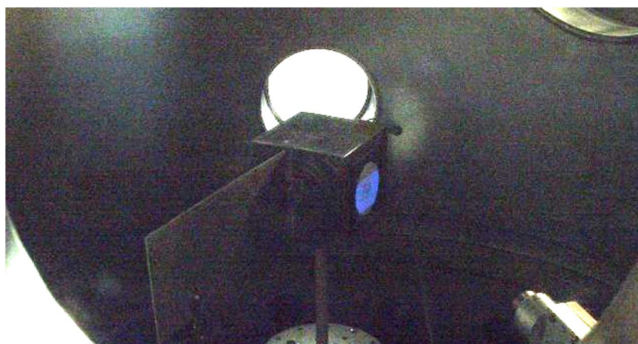
Fig. 10 Wide electron beam for measuring multiple potentials simultaneously.
