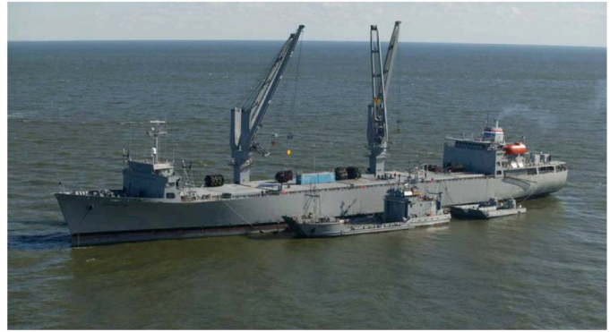
Fig. 1. Cargo Ship Off-Loading Containers Onto Lighter Vessels using Ship-Mounted Boom Cranes.
