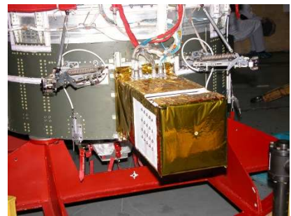
Onboard module, mounted on the SC Glonass-M
