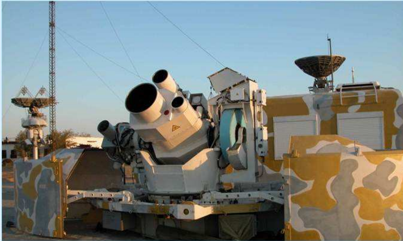
Mobile version of the fourth-generation SLR station (in operation since 2006 at the Baikonur cosmodrome)
